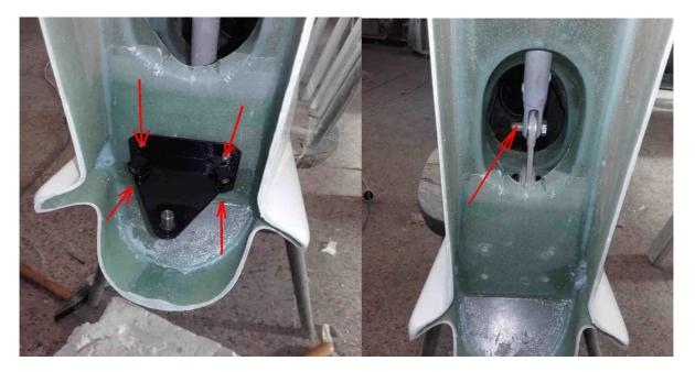
8. Pull the elevator push tube up exposing the bell crank assembly. Make a note of the screw position holding the elevator push tube to the bell crank and number of threads exposed. Remove the screw connecting the bell crank to the elevator push tube (1 M6 screw)
